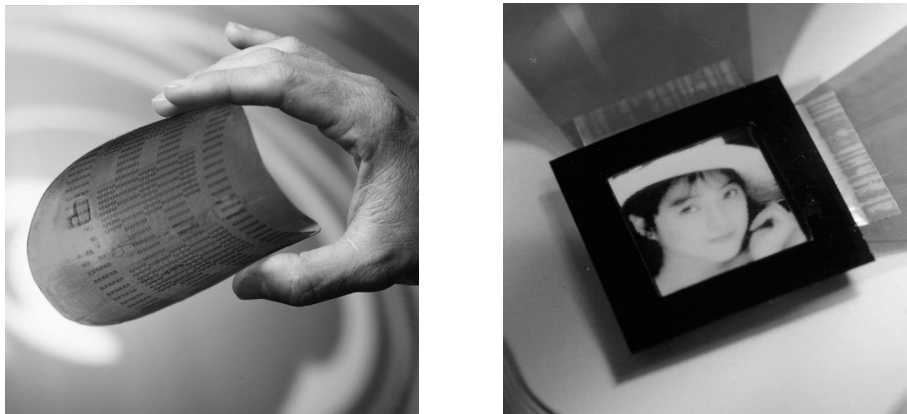
Figure 1.2: On the left: Flexible 6-inch polyimide foil with a variety of components and electronic test circuits. The circuits still operate when the foil is sharply bent. On the right: Example of a display based on polymer LEDs. Photos: Philips Research.
