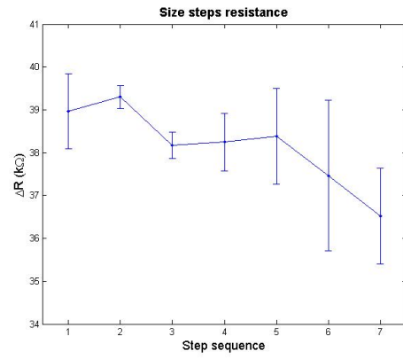
Figure 30: The step size between the resistance levels plotted against the number of the step. The error bars are obtained by calculating the standard deviation of each level separately.
