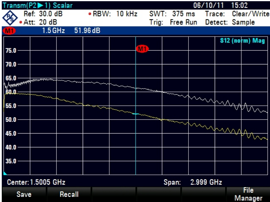
Figure 9: Gain of the amplifier chain (containing three identical amplifiers). The horizontal axis is the frequency of the signal (range: 0 - 3 GHz). The vertical axis is the gain of the three amplifiers (range: 30 - 80 dB). The white line represents the gain at a input power of -50 dBm. Notice that the signal is compressed in the range 0 - 1 Hz, where the maximum input power is exceeded. For the yellow line a 10 dB attenuator is added to the circuit prior to the amplifiers. Notice that the yellow line shows the normal gain of the amplifier chain minus 10 dB. This graph is obtained by using the 'ROHDE&SCHWARTZ FSC3 Spectrum Analyzer'.
