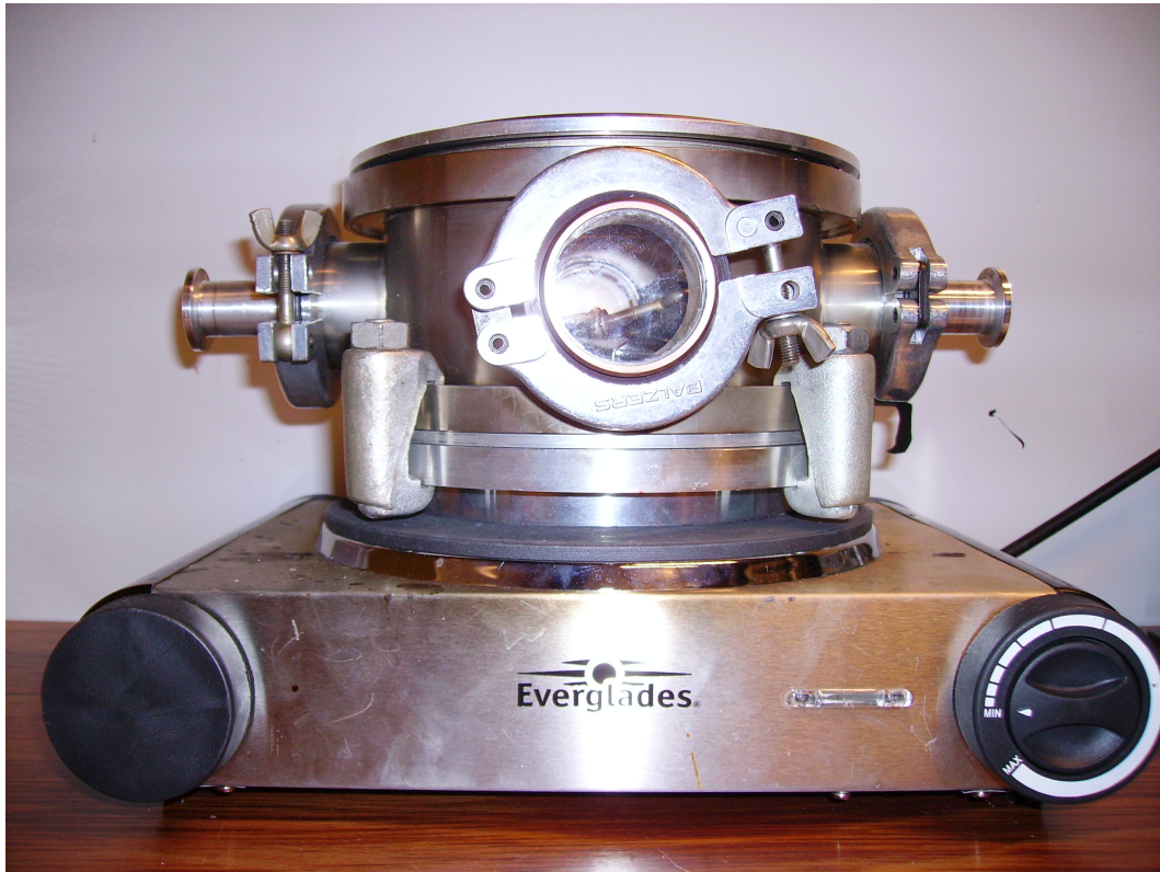
Figure 2.2: Picture of the old oven. The fact that a lot of energy was needed to heat up the oven, combined with the large thermal drift made us decide to build a new oven.
