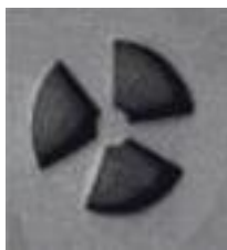
Figure 2.3: Image of a single cavity as seen from the top. The trenches are etched through the upper DBR, the active layer and part of the lower DBR.
